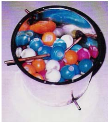
Fig. 5. Photographic view of PCM filled capsules in the storage tank
