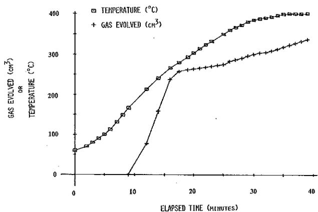
Fig. 2 Result data from a typical pyrolyzation experiment. The temperature is that measured inside the reaction tube, while the gas data is that for net gas evolution when using a dry straw sample of 2.5 grams.
