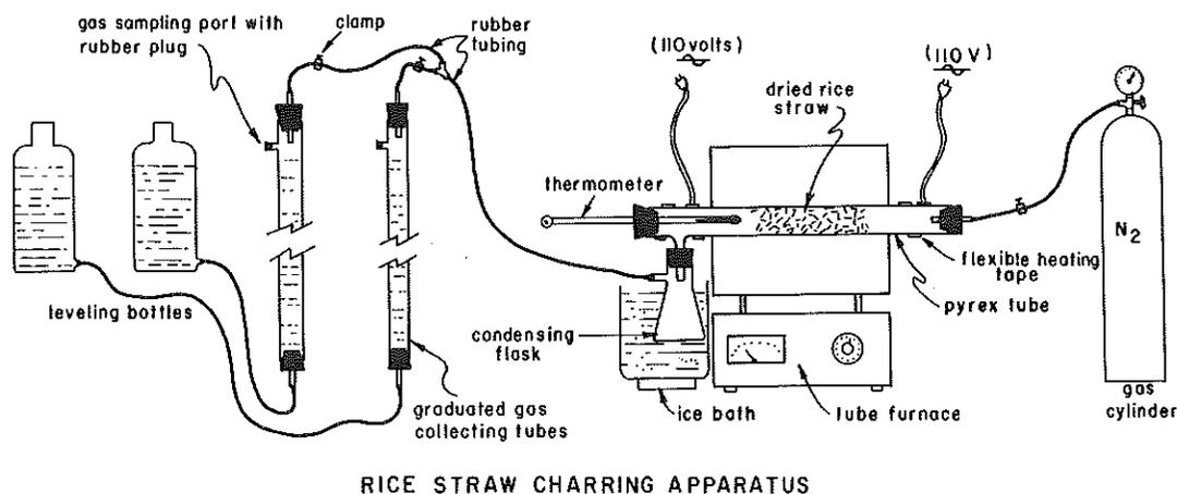
Fig.1 Diagram of the experimental apparatus used in pyrolyzing rice straw.
