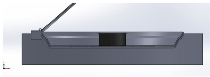
Fig. 1. Cooker with PCM storage with top and bottom trays.
