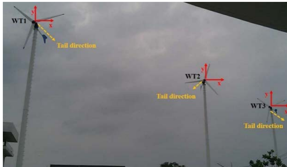
Fig. 20. Direction of wind turbine with usually getting turbulence wind flow in DETC.
