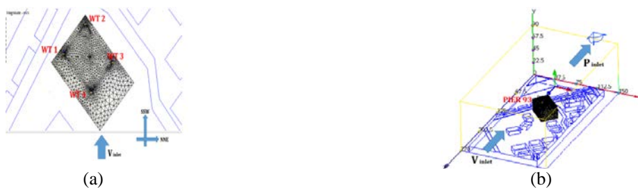
Fig. 17. Boundary condition (a) velocity inlet from SSW direction (b) pressure outlet at outlet side.
