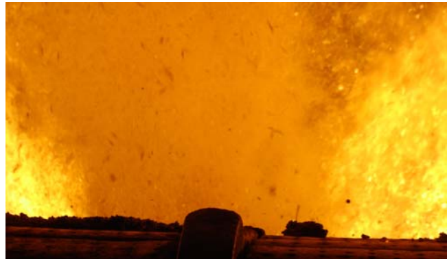
Fig. 17. Image showing the flow of particles at the centre of the furnace (taken from the front wall side) influenced by the tangential air jets
