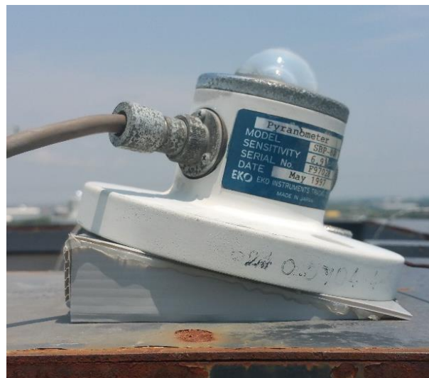
Fig. 8. Pyranometer setup at to measure weather data.
