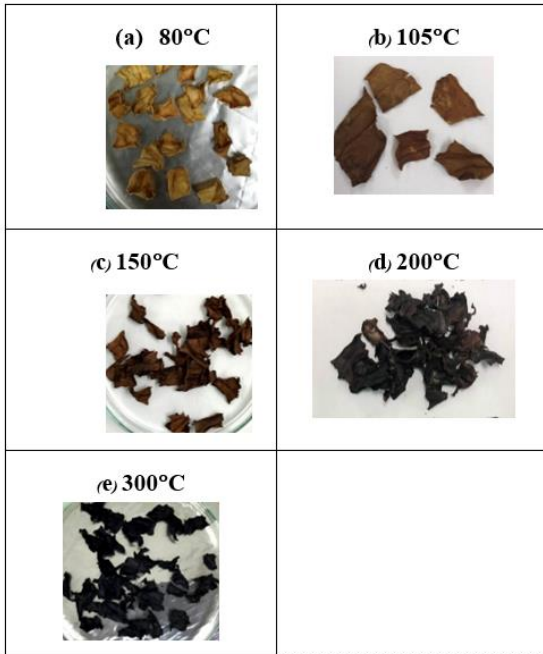
Fig. 5. Physical appearance of cabbage at various temperatures; (a) 80°C (b) 105°C (c) 150°C (d) 200°C (e) 300°C at 15 hours drying time.
