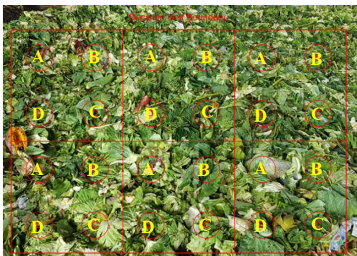
Fig. 1. Organic waste composition by systematic sampling from Nonthaburi city municipality fresh market, Thailand.
