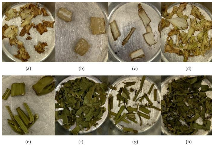
Fig. 4. Physical appearance of organic wastes after drying at 105 °C for 1 h: (a) cabbage; (b) radish; (c) napa cabbage (stalk); (d) napa cabbage (leaf); (e) kale (stalk); (f) kale (leaf); (g) morning glory (stalk); (h) morning glory (leaf).
