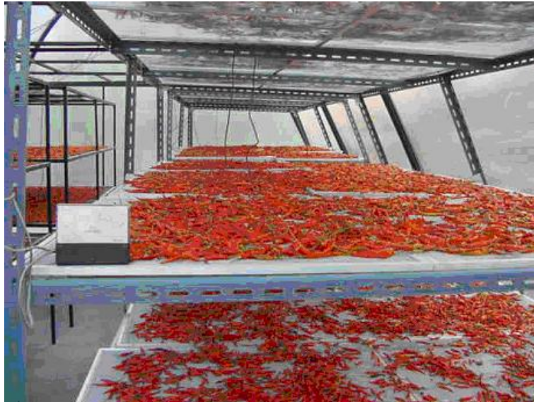
Fig. 3. Chilies on the trays placed on the top, middle and bottom levels of the shelves inside the dryer during the drying experiment
