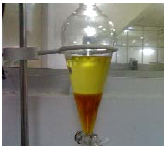
Fig. 2. Separating funnel showing biodiesel-glycerol separation
