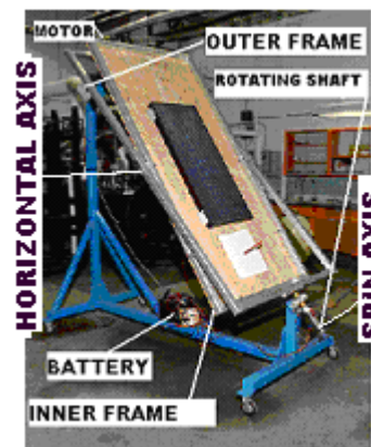
Fig. 19. The solar tracking system.
