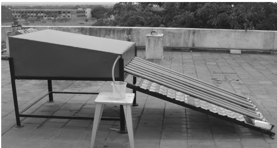
Fig. 2. Photographic view of solar still coupled with evacuated tubes.
