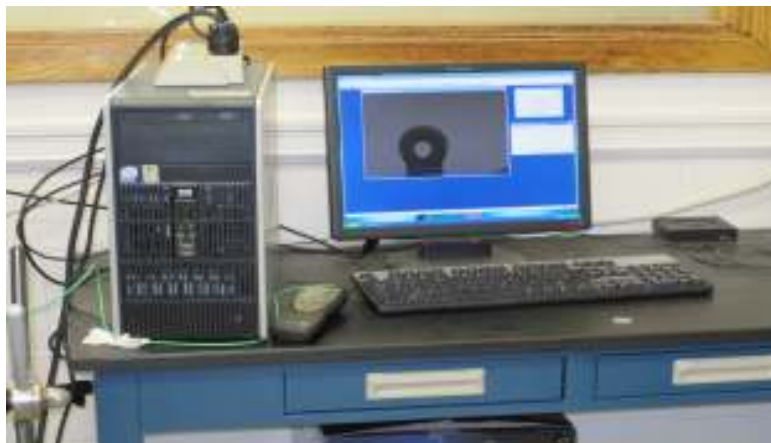
Fig. 2. Pendant drop shape analysis acquiring pendant drop (DSA100 V1.9).
