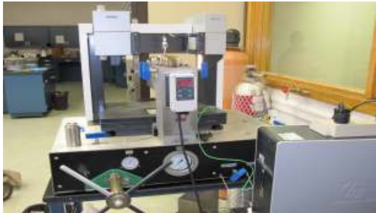
Fig. 1. High-pressure pendant drop equipment (PD-E 1700) and drop shape analysis (DSA100 V1.9).
